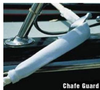
Rubber and vinyl hose can cause problems – edges get sharp and cut as the stuff gets old or if not properly faired in the first place and the hose can cause failure of nylon line by causing heat buildup in the nylon line core when the line is working hard in storm conditions. Rated poorly by Practical Sailor rubber chafe guards contributed to a boat breaking free in a storm – DO NOT USE!
